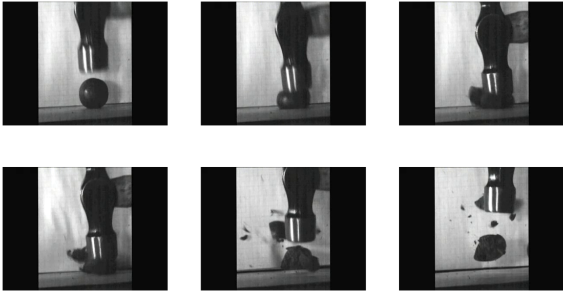
Fig 4 Snapshots of the silly putty hit with a hammer. (Images are snapshots from movies found at http://www.doitpoms.ac.uk/tlplib/glass-transition/index.php )
